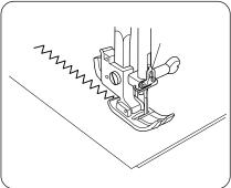
Simple zigzag stitch is widely used for overcasting, applique, sewing on buttons etc.
