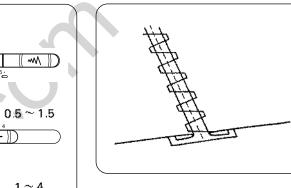
Fold under 1.5cm (1/12") on each fabric edge and press. Pin the two edges to paper 0.3cm (1/8") apart.
