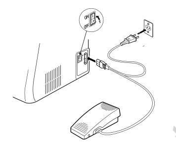
Before connecting the power, make sure the voltage and frequency of your electrical power conform to the machine.
