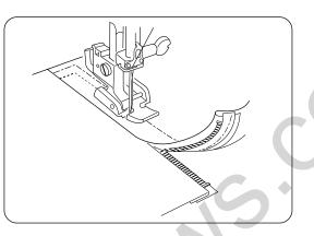
Move the zipper foot to the left pin. Guide the edge of the foot along the zipper teeth and stitch through garment and zipper tape. Stop about 5 cm (2") from the top of the zipper.
