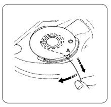
Guide the thread into the notch A on the front side of the bobbin holder. Draw the thread to the left sliding it between the tension spring blades.
