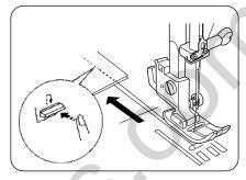
For fastening the ends of seams, press the reverse stitch button and sew several reverse stitches.
