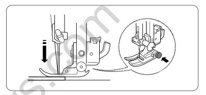
Lower the needle info the fabric at the point where you wish to start sewing. Press the small black button on the zigzag foot with your left hand to "lock" the presser foot to the fabric.
