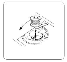
Place the bobbin in the bobbin holder with the thread running counter-clockwise.
