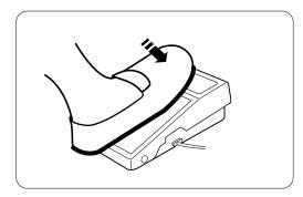
Sewing speed can be varied by the foot control. The harder you press on the control, the faster the machine runs.
