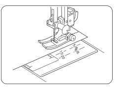
The numbers on the needle plate indicate the distance between the left needle position and the line.
