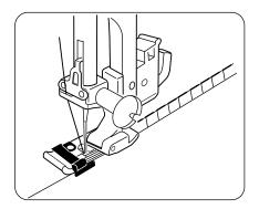
Place the edge of the fabric next to the black prong of foot. The wires on this foot prevent light weight fabric from rolling and creating a ridge. The black prong guides your sewing so the needle falls off the fabric wrapping the threads around the edge to stop raveling.
