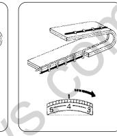
Tighten the needle thread tension by moving the dial to a higher number.
