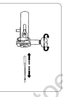
Loosen the needle clamp screw by turning it counter-clockwise.
