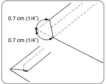
Lower the hemmer foot, then sew by lifting up the edge of the fabric to keep it feeding smoothly and evenly. Trim about 0.7 cm(1/4") from corners as illustrated, to reduce bulk.
