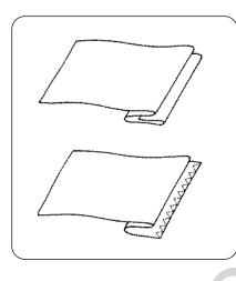
On lightweight fabrics the raw edge can be turned under and pressed. On heavy weight fabrics that ravel, the raw edge should be overcast first.
