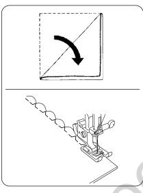
Place the folded edge along the slot of foot. The needle should fall off the edge of the fabric on the right forming a tuck.
