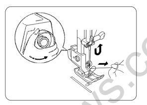
2 Turn the handwheel slowly towards you with your right hand until the needle goes down and continue turning handwheel until the take-up lever is at its highest position.
