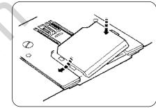
Insert the bobbin Attach the hook cover plate.
