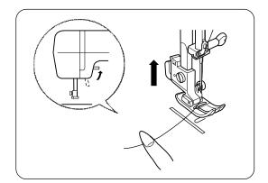
1 Raise the presser foot and hold the needle thread lightly with your left hand.
