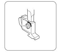
Remove the setscrew by turning the screw counter-clockwise with the screwdriver.
