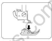
When attaching the presser foot, the pressure dial should always be at position "3".
