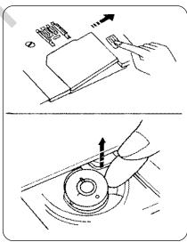
Gently slide the hook cover plate release button to the right, and remove the cover plate. Lift out the bobbin.
