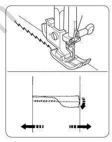
For a 1.5 cm (5/8") seams, use the 2 cm (6/8") marking on the needle plate.
