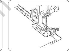
Turn the guide screw and move the sliding guide next to the folded edge. Sew guiding the folded edge along the sliding guide.
