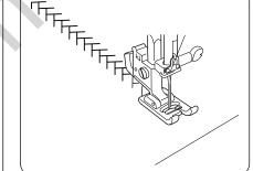
Sew a row of stitches and adjust the thread tension so the needle thread should appear on the reverse side of the fabric. Test the stitch on the actual fabric for the best results. Stitch length of the automatic patterns (No.14 to 23) are preset, so you do not need to select the stitch length for these patterns.
