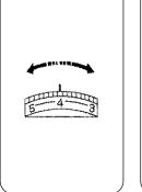
n Set the desired number of the thread tension dial at setting mark. Loosen the needle thread tension by moving the dial to a lower number.
