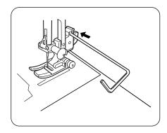
The quiliting guide will help to keep the stitchintg lines straight. Insert the quilter in the opening, and slide it at the desired width.
