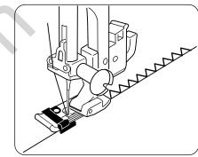
This type of stitch is used on the seam allowance to prevent fabrics from fraying at raw edges. It can be used to finish a hem edge.
