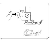
Press the lever on the back of the foot holder.
