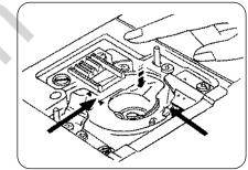
Line up the triangle marks and position the bobbin holder so the notch fits next to the stopper in the hook race.
