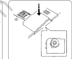
Pull out about 15 cm (6") of thread and attach the hook cover plate.
