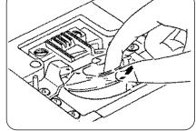
Unplug the machine and remove the presser foot and needle. Remove the screw on the left hand side of the needle plate with the screwdriver. Remove the needle plate. Take out the bobbin. Lift up the bobbin holder and remove it.
