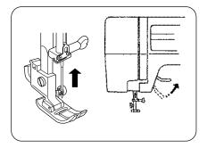
Turn the handwheel toward you to raise the needle to its highest position. Raise the presser foot.
