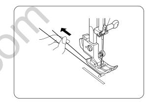
③ Pull 15 cm (6<sup>°</sup>) of both threads back and under the presser foot.
