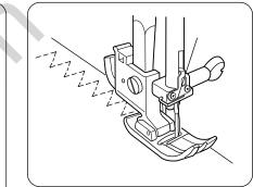
Place the fabric under the presser foot so that the edge will be slightly inside the right hand side of the presser foot. Guide the work so the right hand stitches fall at the edge of the fabric.
