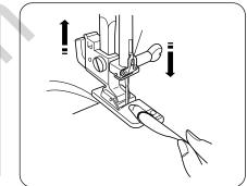
Lower the needle into the fabric and lift the hemmer foot. Insert the folded portion of the fabric into the curl of the hemmer foot.
