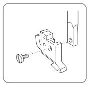
Align the hole in the foot holder with the threaded hole in the presser bar and fit the foot holder screw into the hole. Tighten the screw by turning it clockwise.
