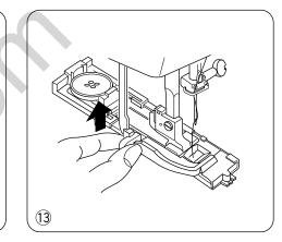
When buttonhole sewing is finished, push the buttonhole lever upward as far as it will go.
