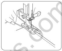
Lower the needle into the fabric at the point where sewing is to begin, then lower the hemmer foot.
