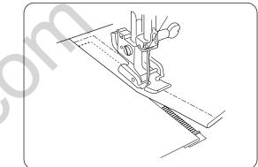
With the needle down in the fabric, raise the foot, remove the basting stitches and open the zipper. Then lower the foot and stitch the remainder of the seam making sure the fold is even.
