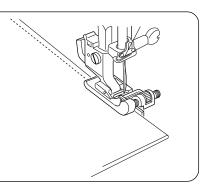
Position the fabric so that the needle pierces 0.1 to 0.2 cm (1/16") inside of folded part and lower the presser foot.
