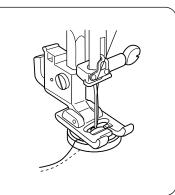
Align the both holes of button with the needle swing, lower the foot and depress the foot control.
