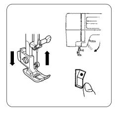
Raise the needle by turning the handwheel toward you and lower the presser foot.
