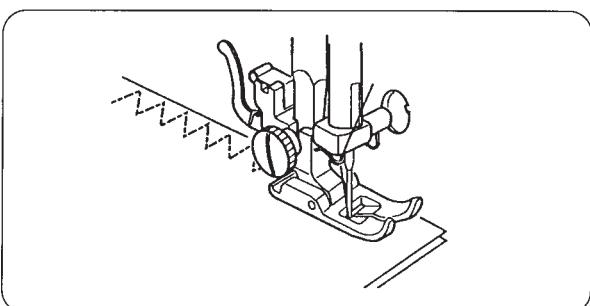
Place the fabric under the presser foot so that the edge is just inside the right edge of the presser foot.
