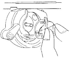
Raise the needle to its highest position and open the hook cover.
