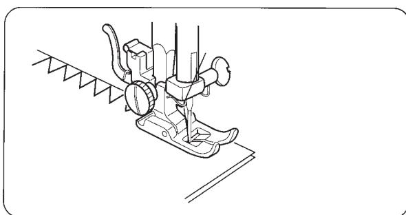
This type of stitch is used on the seam allowance to prevent fabrics from fraying at raw edges.
