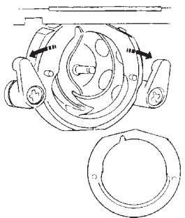
Open the hook race ring holders and remove the hook race ring.
