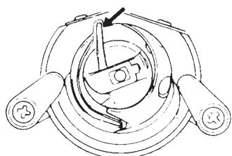
Raise the needle by turning the balance wheel toward you.
