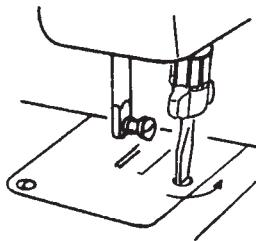
Remove the needle and the presser foot.
