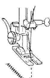
Set the pattern selector dial at “**2**”, sew 5 stitches of bartack and raise the needle from the fabric.
