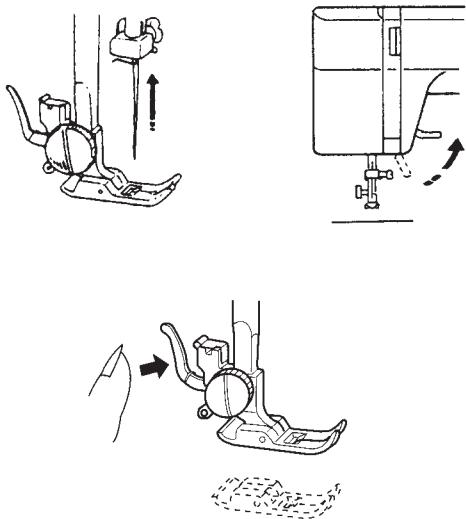
Press the lever on the back of the foot holder.
