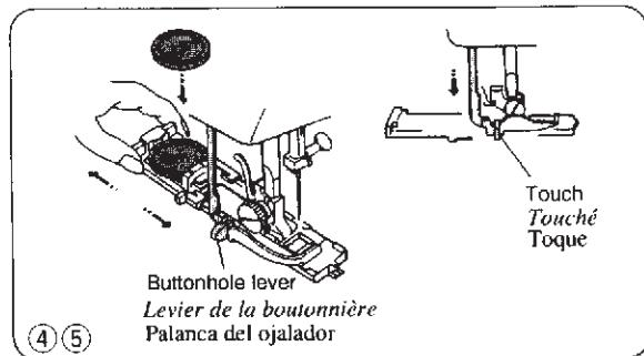
④ Pull the button holder to the back, and place the button in it. Push back the button holder toward you as far as it will go.
