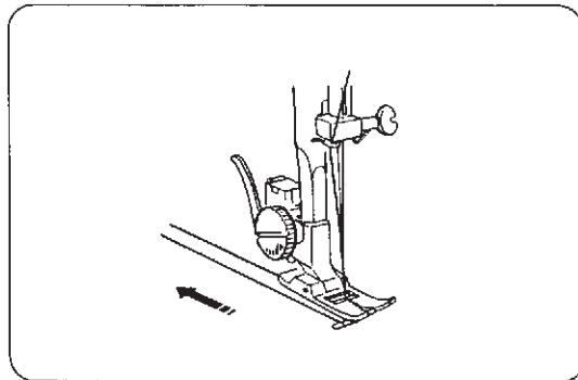
③ Pull 15 cm (6'') of both threads back and under the presser foot.
