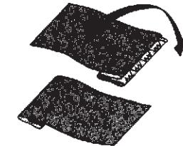
Raise the presser foot and place the fabric under the foot so that the soft fold rests against the wall of hem guide.
