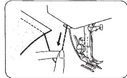
For fastening the ends of seams, press the reverse stitch button and sew several reverse stitches.
