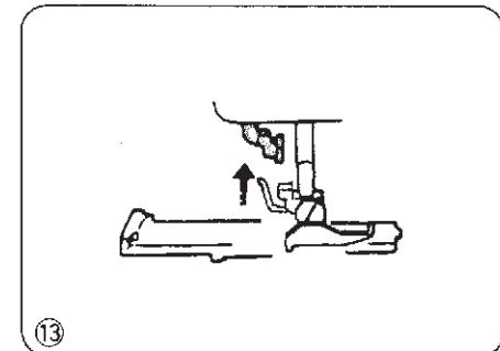
⑬ When buttonhole sewing is finished, push the buttonhole lever upward as far as it will go.
