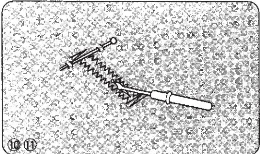
⑩ Cut the both needle and bobbin threads leaving about 10 cm (4") thread ends.
