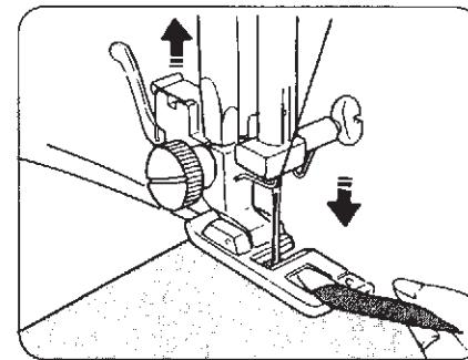
Lower the needle into the fabric and lift the hemmer foot. Insert the folded portion of the fabric into the curl of the hemmer foot.
