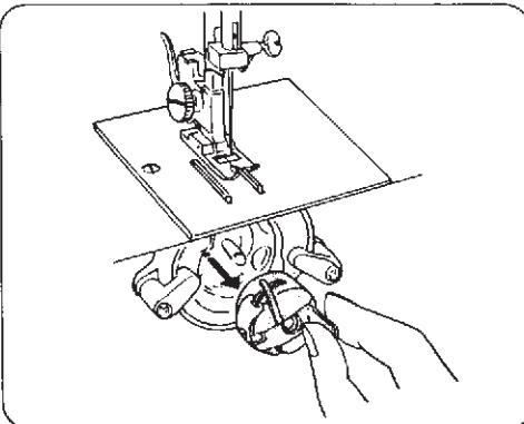
Raise the needle by turning the balance wheel toward you.
