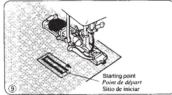
⑨ Sew slowly and stop the machine at the starting point when a buttonhole is completed.
