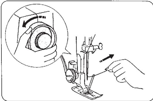
② Turn the balance wheel slowly towards you with your right hand until the needle goes down and continue turning the balance wheel until the take-up lever is at its highest position. Lightly draw up the needle thread forming a loop of the bobbin thread.
