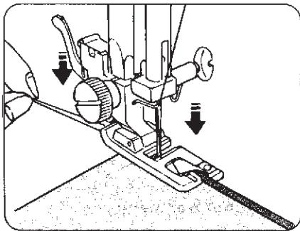
Lower the needle into the fabric at the point where sewing is to begin, then lower the hemmer foot.
