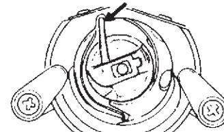
When inserting the bobbin case, place the horn into the recess of the hook race.
