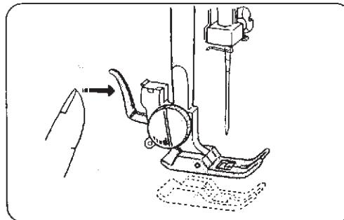
Press the lever on the back of the foot holder. The presser foot will drop off.
