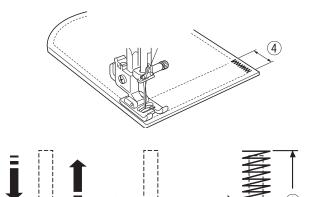
Start the machine and sew until the machine stops automatically. The machine will sew a tacking 1.5 cm (5/8") long. ① 1.5 cm (5/8")
