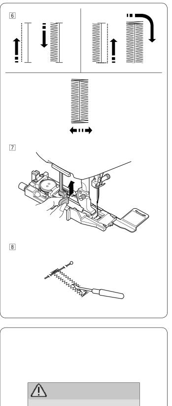
6 The buttonhole is sewn automatically in the sequence shown. When the buttonhole is finished, the machine will stop automatically with the needle in the up position. Press the thread cutter button and remove the fabric.
