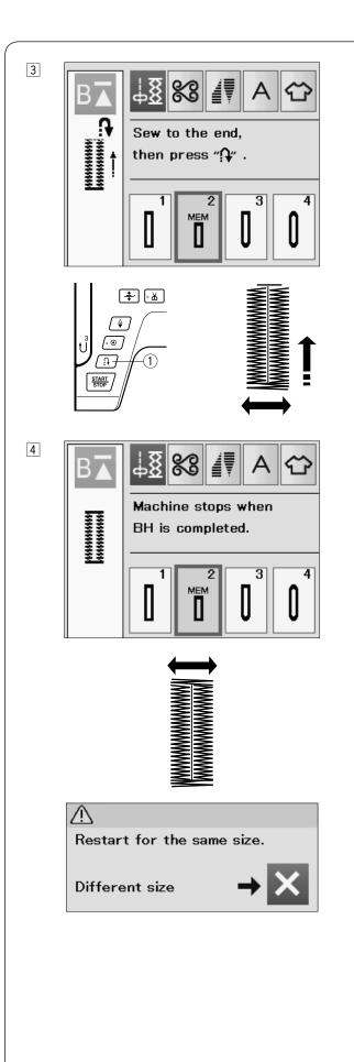
Start sewing again, and the machine sews the front bartack and right side of the buttonhole.
