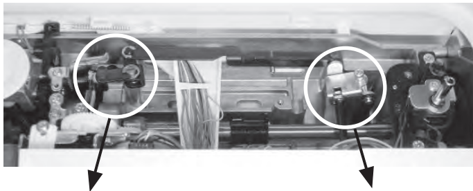
Fig. 2 Presser foot actuator arm bush Thread release plate (for knee lifter)
