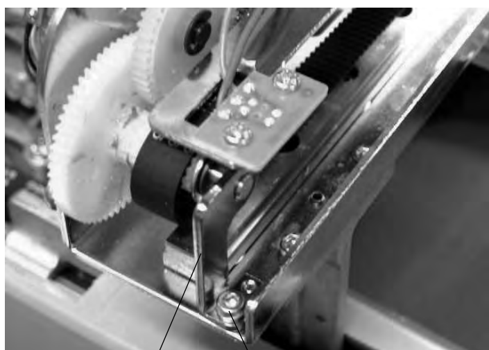
Drive pulley shaft unit
