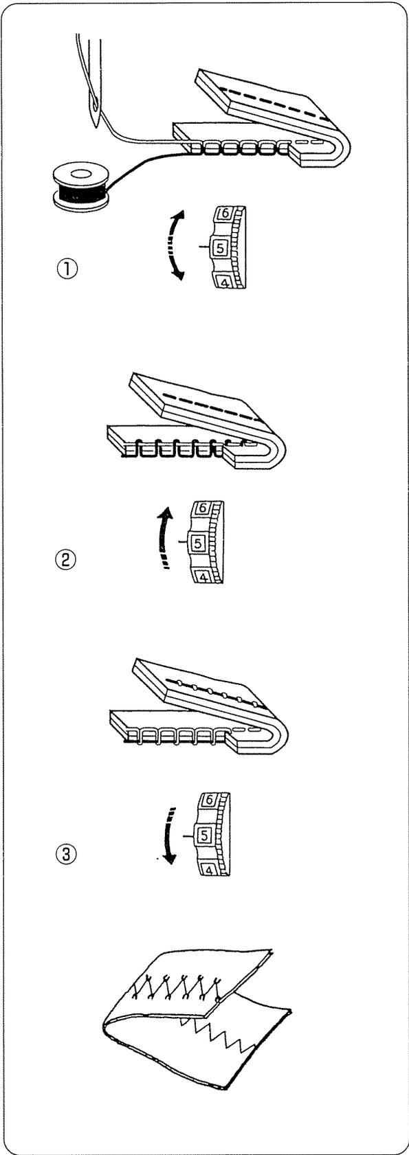
• **Balancing Needle Thread Tension**
