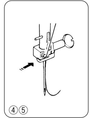
Raise the take-up lever to its highest position by turning the handwheel toward you.
