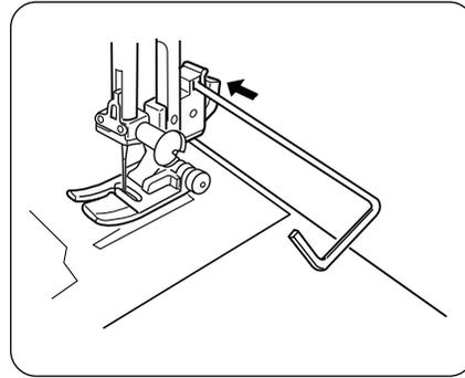
The quilting guide will help to keep the stitching lines straight. Insert the quilter in the opening, and slide it at the desired width.
