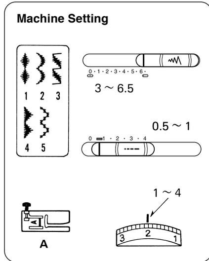
Sew a row of stitches and adjust the thread tension so the needle thread should appear on the reverse side of the fabric.
