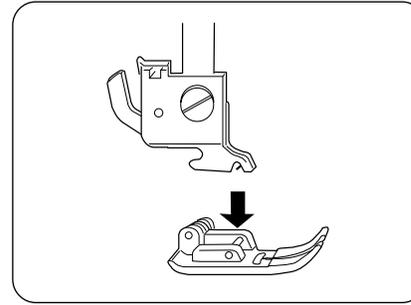
When attaching the presser foot, the pressure dial should always be at position "3". Place the presser foot so the pin on the foot lies just under the groove of the foot holder. Lower the foot holder to lock the foot in place.
