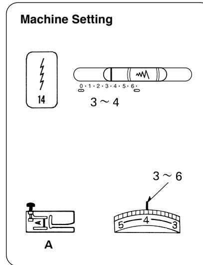
Pattern 14 is a narrow stretch stitch designed to eliminate puckering on knit fabrics and bias seams, while permitting the seam to be pressed completely flat.
