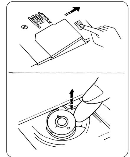
Gently slide the hook cover plate release button to the right, and remove the cover plate. Lift out the bobbin.
