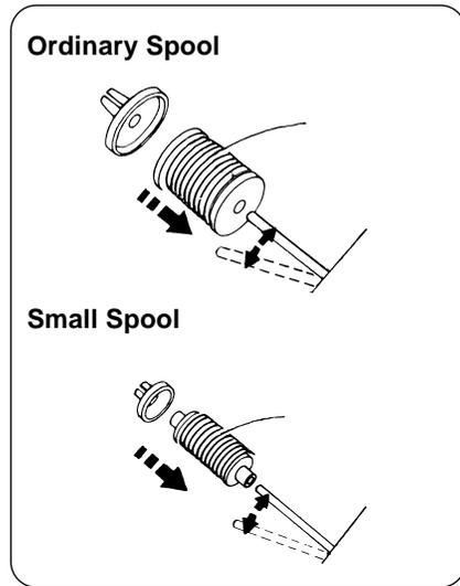
Lift up the spool pin. Place the spool of thread on the spool with the thread coming off the spool as shown. Attach the large spool holder pressing it firmly against the thread spool.
