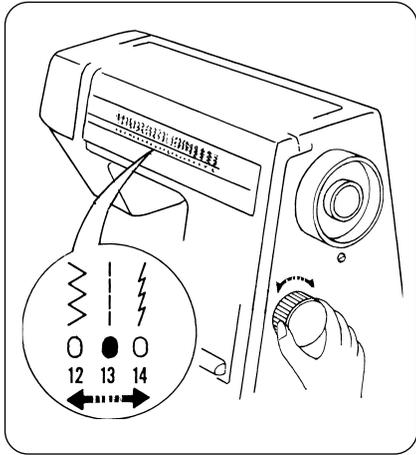
Select the pattern by turning the pattern selector dial and the red signal shows the selected pattern.
