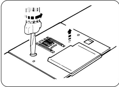
Unplug the machine and remove the presser foot and needle. Remove the screw on the left hand side of the needle plate with the screwdriver. Remove the needle plate.
