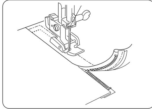
Move the zipper foot to the left pin. Guide the edge of the foot along the zipper teeth and stitch through garment and zipper tape. Stop about 5 cm (2") from the top of the zipper.
