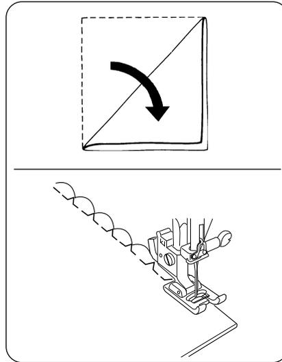
Place the folded edge along the slot of foot. The needle should fall off the edge of the fabric on the right forming a tuck.
