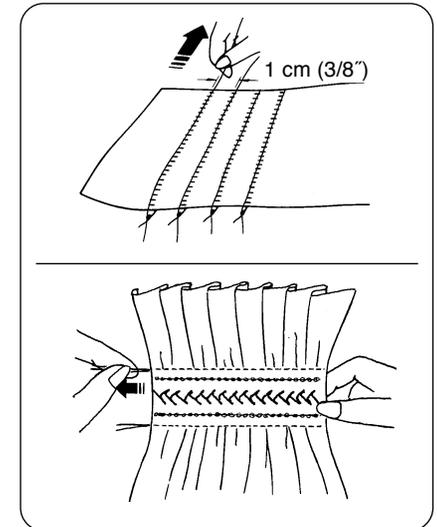
With the stitch length control at “4”, sew straight lines 1 cm (3/8”) apart across the area to be smocked. Knot the threads along the edge. Pull the bobbin threads and distribute gathers evenly. Sew pattern stitches between the straight seams. Pull out the gathering stitches.
