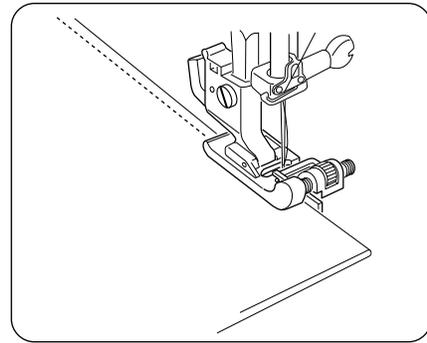
Position the fabric so that the needle pierces 0.1 to 0.2 cm (1/16") inside of folded part and lower the presser foot.
