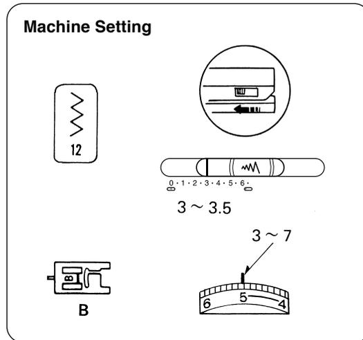
Tape the button over the placement mark. A pin can be placed on top of the foot to from a shank. Before lowering the foot, test the needle swing making sure the needle drops in each hole. Adjust the stitch width if necessary. Lower the foot.
