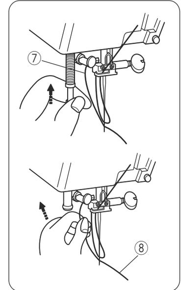
Raise the threader knob slowly. The thread loop is pulled up through the needle eye. Pull the thread loop to remove the thread end to the rear.
