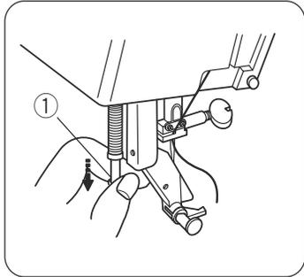
Raise the needle to the highest position. Lower the presser foot.
