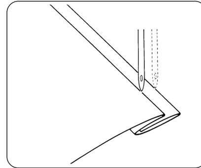
Position the fabric on the machine so that the needle just pierces the folded part of the fabric when the needle comes over to the extreme left side.
