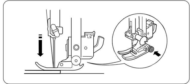
Lower the needle into the fabric at the point where you wish to start sewing. Press the small black button on the zigzag foot with your left hand to “lock” the presser foot to the fabric.
