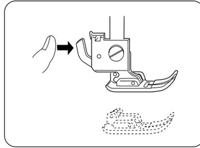
Press the lever on the back of the foot holder. The presser foot will drop off.
