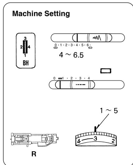
\* Set the stitch width in accordance with the thickness of the cord used.
