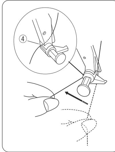
Draw the thread to the left into the groove on the back.
