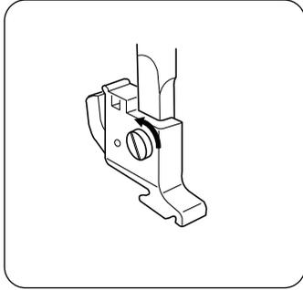
Remove the thumb screw by turning the screw counter-clockwise with the screwdriver.
