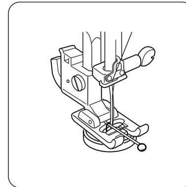
To strengthen the shank, cut the threads leaving a 20 cm (8") tail. Bring the needle thread down through the hole in the button and wind it around the shank. Draw the thread to the wrong side of fabric and knot.
