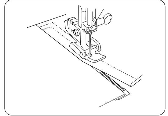
With the needle down in the fabric, raise the foot, remove the basting stitches and open the zipper. Then lower the foot and stitch the remainder of the seam making sure the fold is even.
