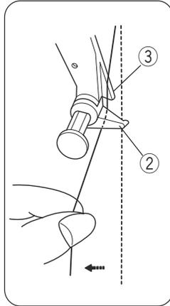
Pass the thread between the horn and triangle as shown.
