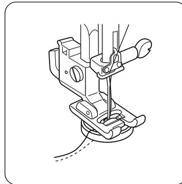
Align the both holes of button with the needle swing, lower the foot and depress the foot control.
