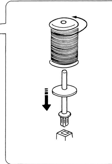
The additional spool pin is used to wind extra bobbins without unthreading the machine. To use, insert the additional spool pin in the hole. Place the felt and the spool on the pin.
