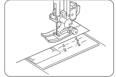
The numbers on the needle plate indicate the distance between the left needle position and the line.
