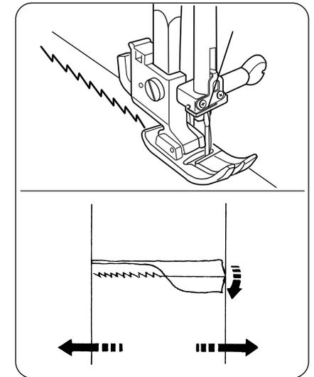
For a 1.5 cm (5/8") seams, use the 2 cm (6/8") marking on the needle plate.
