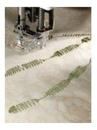
stitch, then while the machine is still running, press against the knee lifter to widen your stitch to a 9mm zigzag. Release pressure to gradually return to a straight stitch for a tapered finish. This advanced feature opens up amazing new possibilities for creation expression with free motion quilting, thread painting, raw edge appliqué, free motion monogramming, and more.
