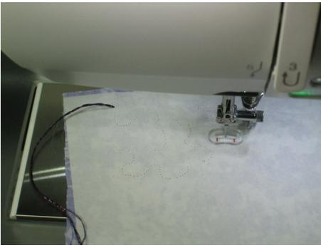
*Note: You are in control of the direction of the stitches and the stitch length. The faster you move the fabric the longer the stitch length. You will need to practice to find the speed of the machine that best works with the speed you move the fabric.*
