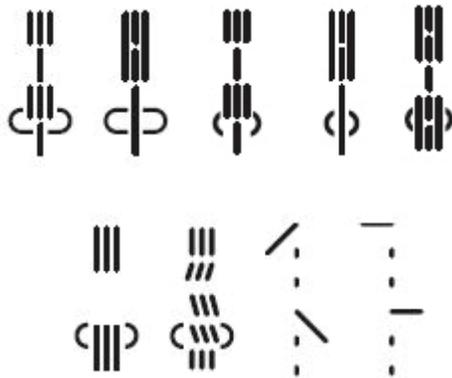
3. If your machine does not have automatic thread tension settings, tighten the needle thread tension.
