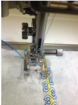
11. Once completed, press the needle/ up down button to pull-up the bobbin thread.
