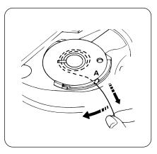
Guide the thread into the notch A on the front side of the bobbin holder. Draw the thread to the left sliding it between the tension spring blades.
