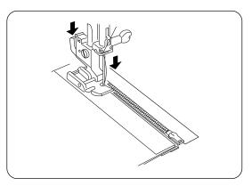
Attach the zipper foot with the pin on the right hand side. Lower the zipper foot.
