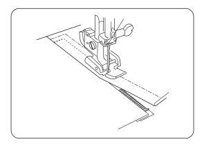
With the needle down in the fabric, raise the foot, remove the basting stitches and open the zipper. Then lower the foot and stitch the remainder of the seam making sure the fold is even.
