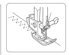
Place the fabric under the presser foot so that the edge will be slightly inside the right hand side of the presser foot. Guide the work so the right hand stitches fall at the edge of the fabric.
