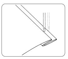
Position the fabric on the machine so that the needle just pierces the folded part of the fabric when the needle comes over to the extreme left side.
