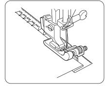
Turn the guide screw and move the sliding guide next to the folded edge. Sew guiding the folded edge along the sliding guide.
