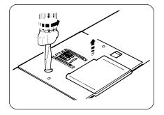
Unplug the machine and remove the presser foot and needle. Remove the screw on the left hand side of the needle plate with the screwdriver. Remove the needle plate.
