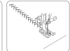
Sew a row of stitches and adjust the thread tension so the needle thread should appear on the reverse side of the fabric.
