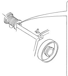
Lift up the spool pin. Place the spool of thread on the spool with the thread coming off the spool as shown.
