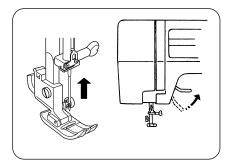
Turn the handwheel toward you to raise the needle to its highest position. Raise the presser foot. Press the lever on the back of the foot holder. The presser foot will drop off.
