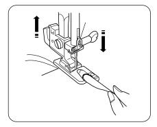
Lower the needle into the fabric and lift the hemmer foot. Insert the folded portion of the fabric into the curl of the hemmer foot.
