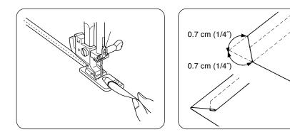
Lower the hemmer foot, then sew by lifting up the edge of the fabric to keep it feeding smoothly and evenly. Trim about 0.7 cm(1/4") from corners as illustrated, to reduce bulk.
