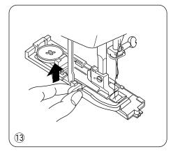
When buttonhole sewing is finished, push the buttonhole lever upward as far as it will go.
