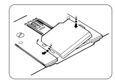
Insert the bobbin Attach the hook cover plate.
