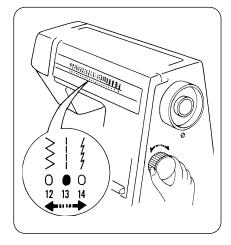
Select the pattern by turning the pattern selector dial and the red signal shows the selected pattern.
