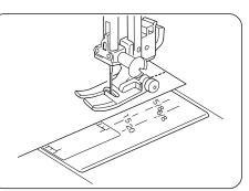
The numbers on the needle plate indicate the distance between the left needle position and the line.
