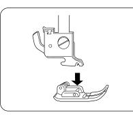
When attaching the presser foot, the pressure dial should always be at position "3".
