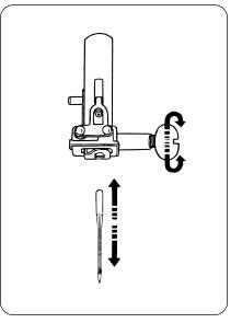
Loosen the needle clamp screw by turning it counter-clockwise.
