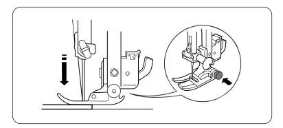
Lower the needle info the fabric at the point where you wish to start sewing. Press the small black button on the zigzag foot with your left hand to "lock" the presser foot to the fabric.
