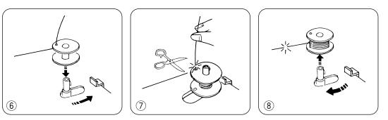
(6) Put the bobbin on the bobbin winder spindle, and push it to the right.
