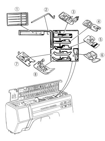
Each presser foot and pocket is lettered for easy identification and storage. To achieve optimum sewing results, use the foot recommended for each sewing technique.
