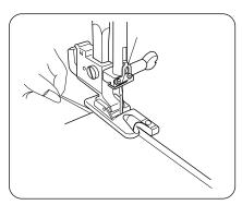
Lower the needle into the fabric at the point where sewing is to begin, then lower the hemmer foot.
