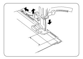
Sew through fold and zipper tape. Stop just before the zipper foot reaches the slider on the zipper tape.
