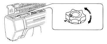
The pressure dial should be set at "3" for regular sewing. Reduce the pressure to "2" for appliques.
