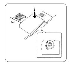
Pull out about 15 cm (6") of thread and attach the hook cover plate.
