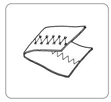
To obtain better zigzag stitches, the needle thread tension should be slightly weaker than in the case of straight sewing. The needle thread should appear slightly on the reverse side of the fabric.
