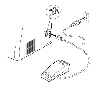
Before connecting the power, make sure the voltage and frequency of your electrical power conform to the machine.
