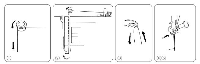
Raise the take-up lever to its highest position by turning the handwheel toward you. Raise the presser foot with the presser foot lifter and thread in the order from (1) to (5).
