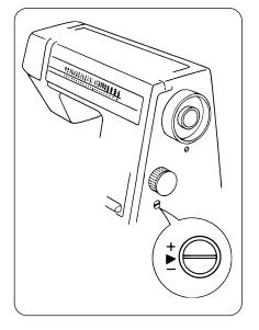
If patterns are uneven when sewing with a particular fabric, adjust them with the feed balance dial.
