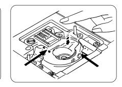
Line up the triangle marks and position the bobbin holder so the notch fits next to the stopper in the hook race.
