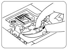
Take out the bobbin. Lift up the bobbin holder and remove it.
