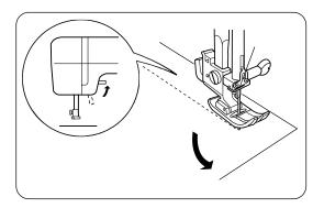
Stop the machine and bring the needle down into the fabric by turning the handwheel. Raise the presser foot.
