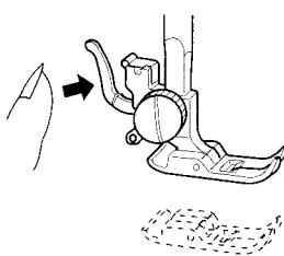
Press the lever on the back of the foot holder.
