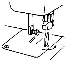
Remove the needle and the presser foot.
