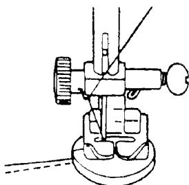
A pin can be placed on top of the foot to form a shank.
