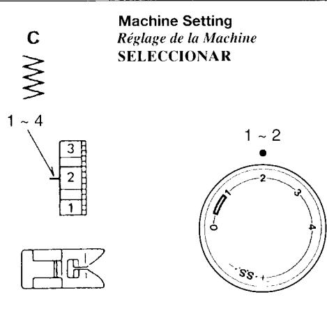
This type of stitch is used on the seam allowance to prevent fabrics from fraying at raw edges.
