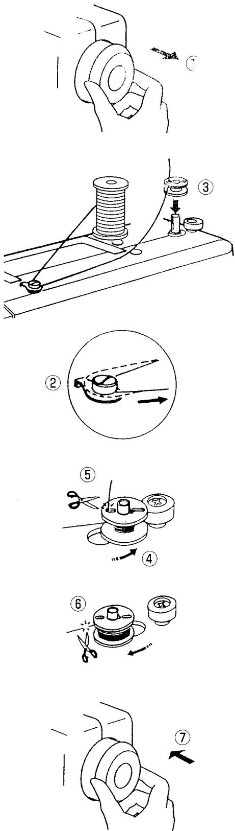
① Pull the handwheel out.
