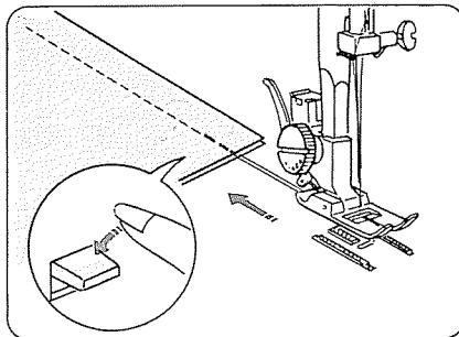
For fastening the ends of seams, press the reverse stitch lever and sew several reverse stitches.
