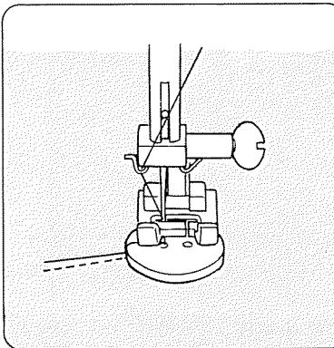
Set the pattern selector at “”. Align the both holes of the button with the slot of the foot and place the left hole of the button just below the needle point. Lower the foot and turn the pattern selector until the needle point comes just above the right hole of the button. Sew about five stitches and raise needle. Set the pattern selector at “” again and sew a few stitches to lock thread.
