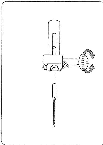
Loosen the needle clamp screw by turning it toward you.
