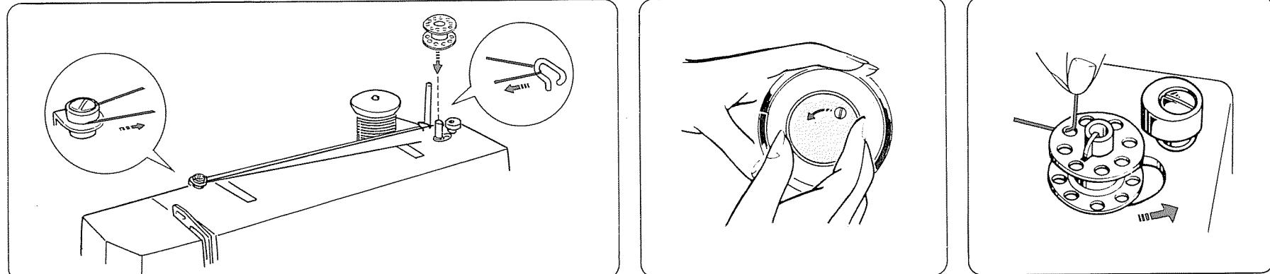
Draw the thread from the spool. Pass the thread through the top cover thread guide. Guide the thread around the bobbin winder thread guide. Insert the thread through the hole in the bobbin, threading from inside to outside. Put the bobbin on the bobbin winder spindle, and push it to the right.
