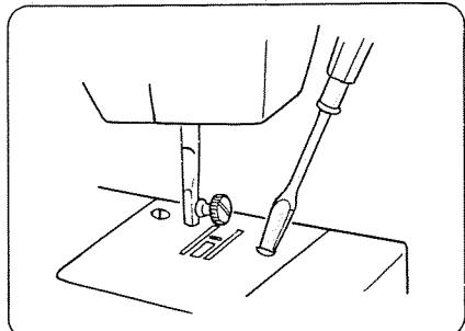
Remove the needle and the presser foot.
