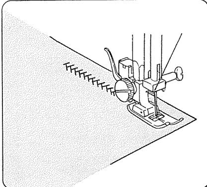
When forward and reverse feeds become unbalanced depending upon the type of fabric, correct the balance by turning the stitch length dial as follows:
