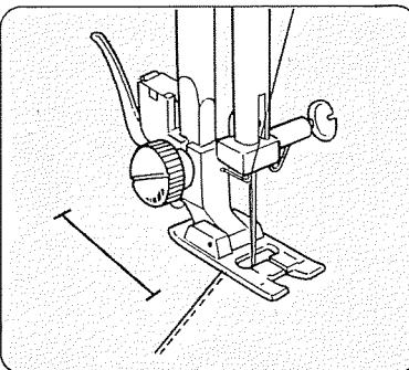
Set the pattern selector dial at “ ”. Slide both threads to the left. Lower the needle into the garment where the buttonhole is to start, and lower the foot.
