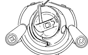
When inserting the bobbin case, place the horn into the recess of the hook race.
