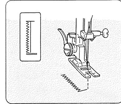
Set the pattern selector dial at “ ”, sew 5 stitches of bartack and raise the needle from the fabric.
