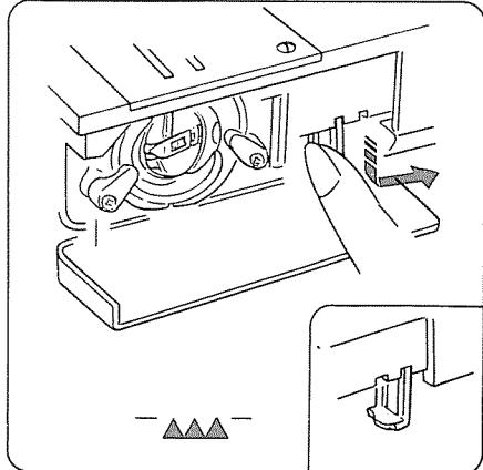
For dropping the feed dogs, press down the lever and move it to the direction of arrow as illustrated.
