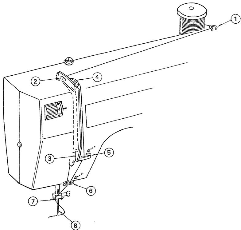
Raise the thread take-up lever to the highest position by turning the balance wheel towards you.
