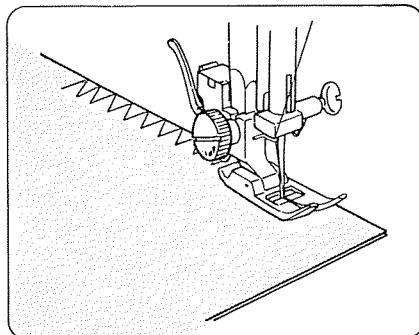
This type of stitch is used on the seam allowance to prevent fabrics from fraying at raw edges.
