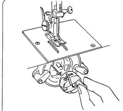
Raise the needle by turning the balance wheel toward you.
