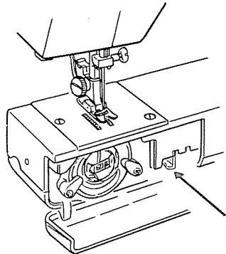
The drop feed lever is located in the hook area.
