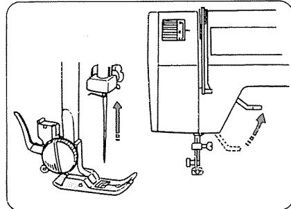
Turn the balance wheel toward you to raise the needle to its highest position. Raise the presser foot.
