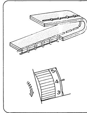
Tighten the needle thread tension by moving the dial to a higher number.
