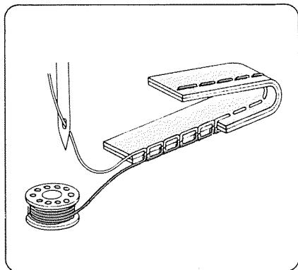
The needle thread and the bobbin thread should interlock in the center of two layers of fabric in straight seams.
