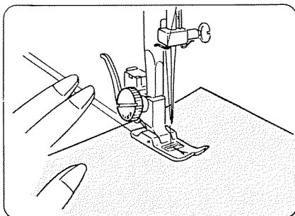
Raise the presser foot and position the fabric next to a stitching guide line on the needle plate.
