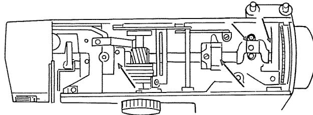
Turn the screw to the left and remove the face plate.
