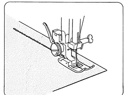
The stitch is sewn with two stitches forward and one stitch backward forming a seam that does not rip easily.
