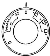
Raise the needle above the fabrics and select the desired pattern at the setting mark by turning the pattern selector dial.
