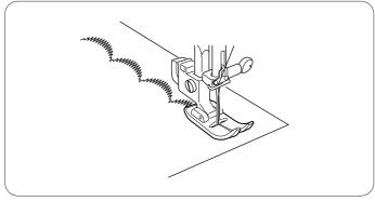
Determine the appropriate stitch density by test sewing. For a delicate appearance on fabric such as chiffon, use a single layer with a tear-away backing, if necessary. Reduce the needle thread tension slightly to achieve the better result.
