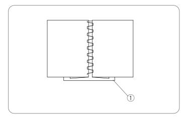
Use this stitch to join two pieces of fabric to create an open work appearance, and add design interest. Fold under each fabric edge 1/2" (1.3 cm) and press. Pin the two edges to a piece of paper or tear-away backing 1/8" (0.3 cm) apart.
