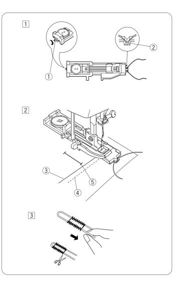
1 With the buttonhole foot raised, hook the filler cord on the spur at the back of the foot.
