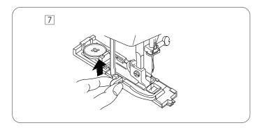
7 When buttonhole sewing is finished, push the buttonhole lever up as far as it will go.
