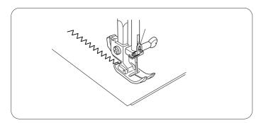
Simple zigzag stitching is widely used for overcasting, sewing on buttons etc.
