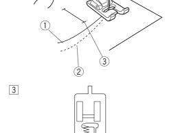
3 Sew the front bartack and left row to the desired length then stop the machine.
