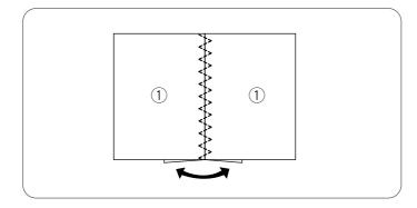
Place two layers of the fabric with the right side together. Seam along the edges with the straight stitch. Open fabrics flat and fold each seam allowances.
