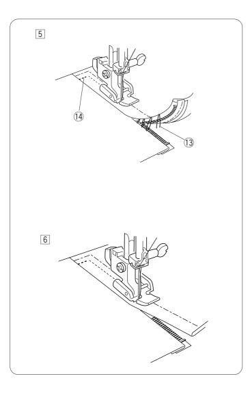
5 Raise and release the foot, and re-attach it with the left side pin.
