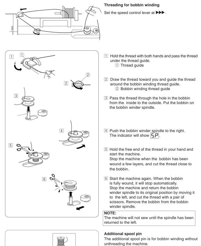
Insert the additional spool pin into the hole.
