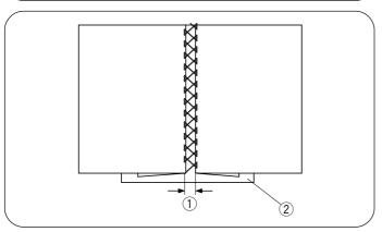
Use this stitch to join two pieces of fabric to create an open work appearance and add design interest. Fold under each fabric edge  $5/8^{\circ}$  (1.5 cm) and press. Pin the two edges to paper or tear backing  $1/8^{\circ}$  (0.3  $\sim$  0.4 cm) apart. Sew slowly, guiding the fabric so the needle catches the folded edge on each side.
