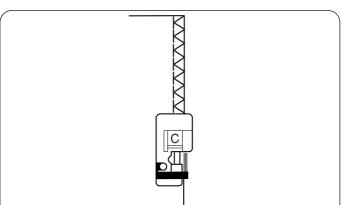
This stitch pattern combines the straight and the zigzag stitches, using the overedge foot, to seam and overcast in one step.
