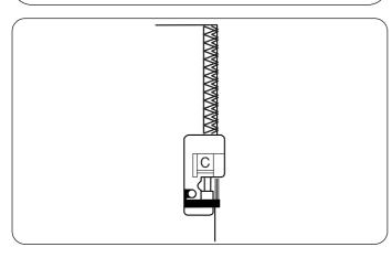
This stitch can be used for sewing fabrics that tend to fray extensively such as linens and gabardines. Two rows of zigzag stitches are simultaneously sewn over the edge to insure that your seams will not ravel. Adjust the thread tension so both the needle and bobbin threads meet at the edge of the fabric.
