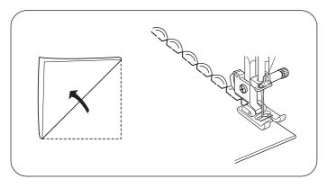
Use a lightweight fabric (tricot, for example). Fold the fabric as shown and stitch on the fold. Allow the needle to just clear the folded edge to create a shelled edge. You may need to increase the needle thread tension slightly.
