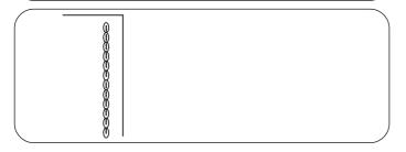
This strong, durable stitch is recommended when both elasticity and strength are necessary in order to insure comfort and durability. Use it to reinforce areas such as crotch and armhole seams. Also use for extra reinforcement when constructing items such as backpacks.
