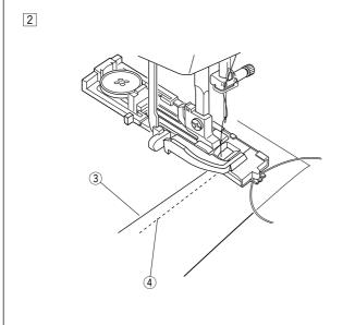
2 Start the machine and sew the buttonhole. Each side of the buttonhole and the bartacks will be sewn over the cord.
