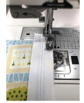
5. Use the zipper short-cut (stored in the S9) to quickly move the needle position to the left side:
