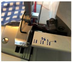
• Lift presser foot and gently pull fabric to the rear, removing it from stitch "finger" on needle plate.
